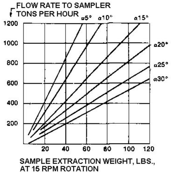
EXTRACTION WEIGHT AT OTHER ROTATION RATES IS PROPORTIONAL TO RPM. ADJUST WEIGHT OF SAMPLE ACCORDING TO RPM.
